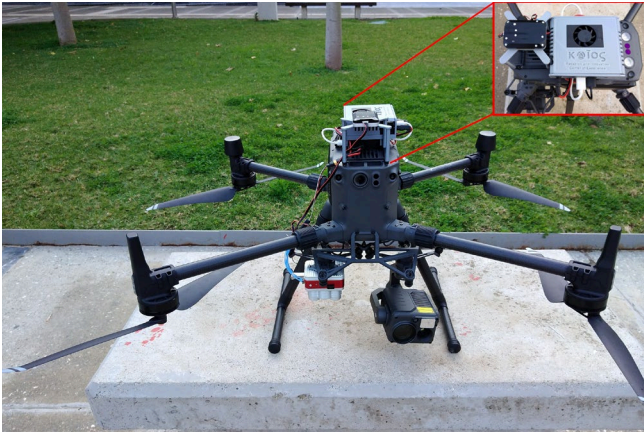
Fig. 1: Equipment for implementing ICARUS inspection platform, consisting of the DJI Matrice 300 RTK UAV, the multi-sensor (RGB and thermal) DJI Zenmuse H20T camera (right downward gimbal), the MicaSense Altum multispectral camera (left downward gimbal) and the NVIDIA Jetson Xavier NX embedded platform (top of UAV; figure inset).
