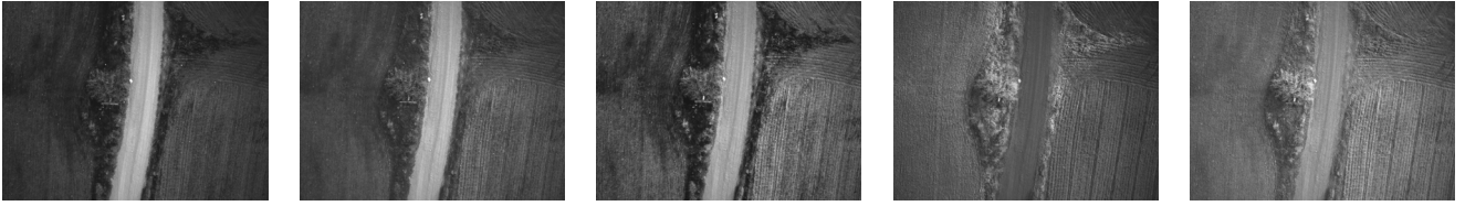
Fig. 5: Multispectral imaging of the power line corridor. From left to right the blue (475±32nm), green (560±27nm), red (668±14nm), red edge (717±12nm), and near infrared (842±57) channels are shown [35].
