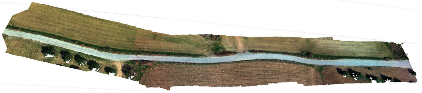
Fig. 7: Dense 3D model resulted by implementing photogrammetric algorithms on the multispectral dataset.
