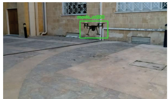
Fig. 2: Detection of a DJI M210 drone.
